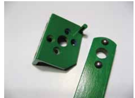
The handle lever with ball bearings; and bracket plate with locking holes
