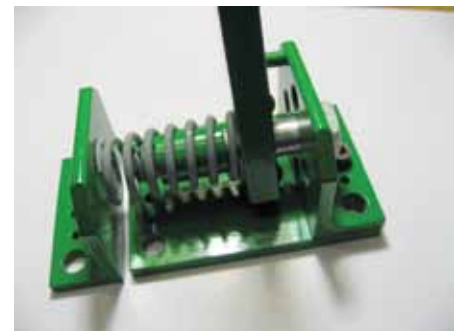
The partially assembled mounting bracket
