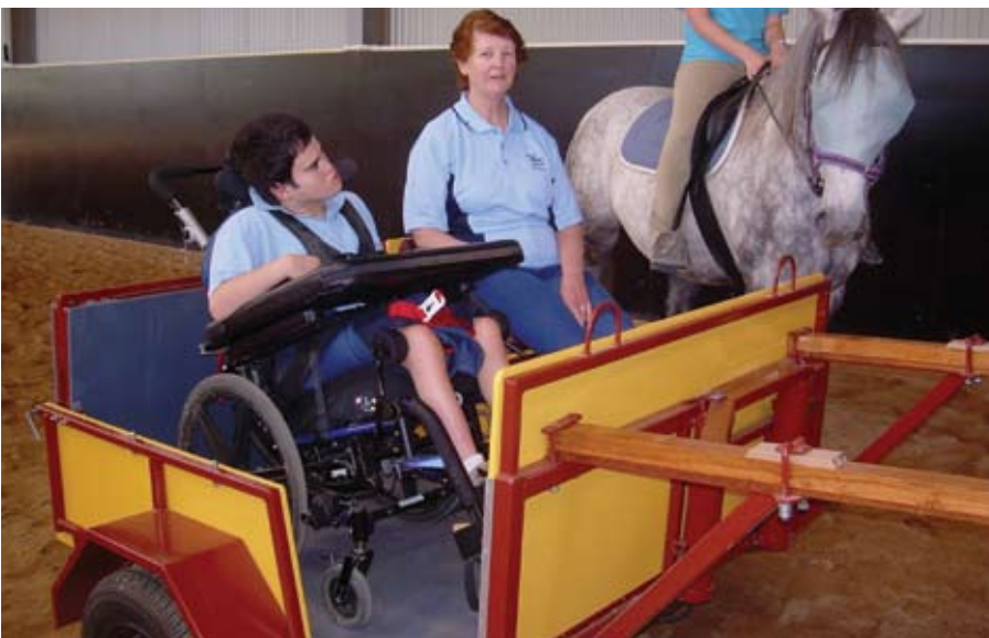
Top: The cart with the three seats in place. The swindle bar is visible between the wooden shafts at the front. Centre: The ramp folded down for wheelchair access. Below: The wheelchair in place on the cart, with two of the seats removed.
